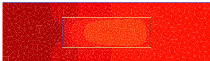
$$\omega = \frac{\omega_d}{3}, \text{ Pressure is nearly uniform}$$
