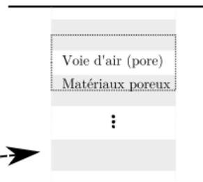
HVAC Silencers are most often made of parallel baffles of porous material (rockwool)
