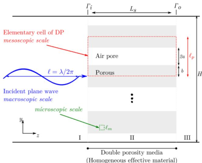
In each domain, only the fundamental mode is taken into account. The pressure field fulfils the 1D Helmholtz equation according to  $z$  direction ( $e^{i\omega t}$ ).
