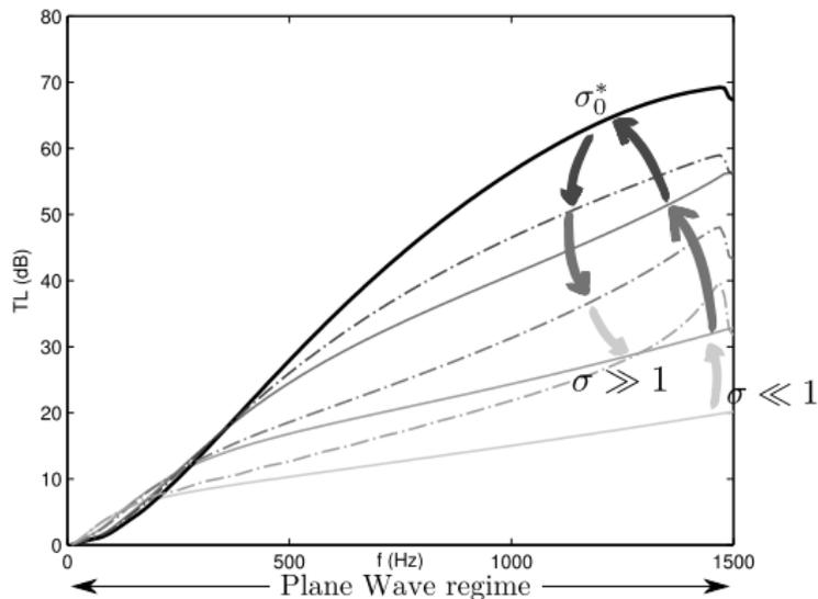
An optimal value exists and corresponds to the best compromise for the fundamental mode attenuation.
