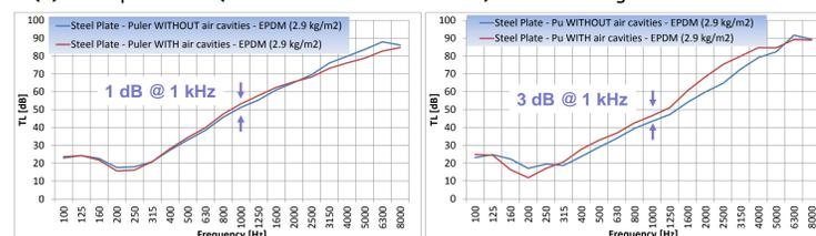
Figure 2: Air cavities effect on Transmission Loss for PU and Puler foams
